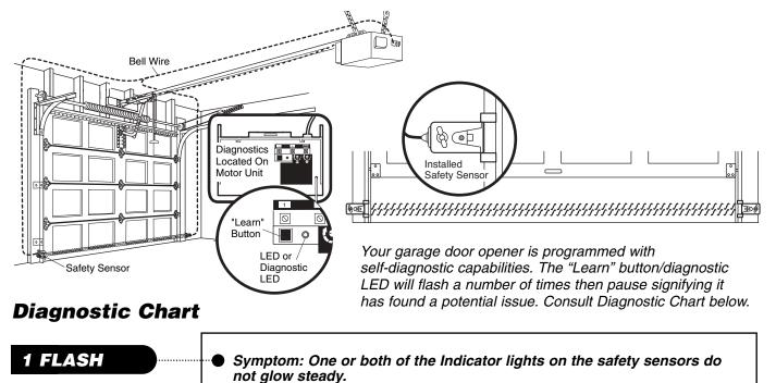
Safety sensors wire open (broken or disconnected).
